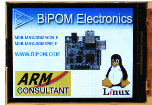
MINI-MAX/ARM9260-E Ethernet, 2 USB ports, ATMEL AT91SAM9260
